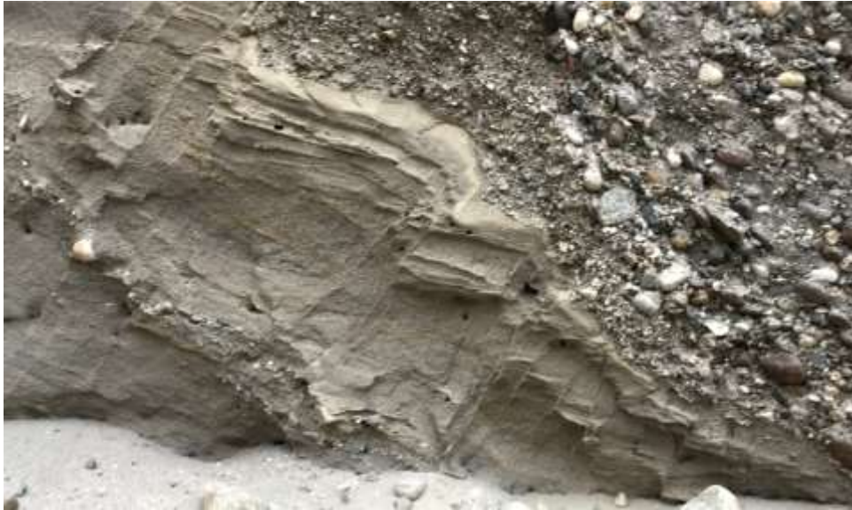
Photo 8-23 Development of Micro Faults in Sand.
