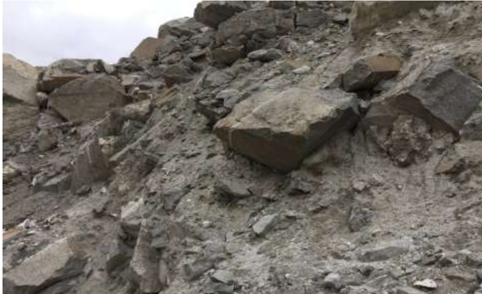
Photo 7-7 Fill Material (Boulder and Gravels) in Slided Mass.
