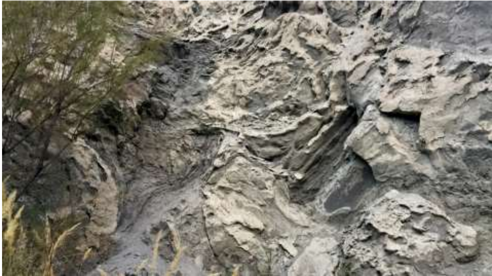
Photo 8-13 Sheared and Smeared Clayey Silt at Sarat Village.
